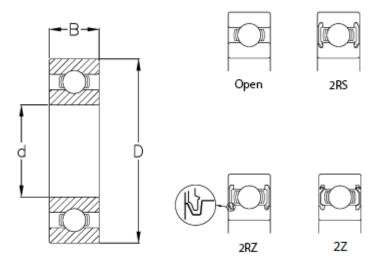
B = 12 Ball grade = 5 C (KN) = 9.36 C0 = 5.1 d = 20 D = 42 Max rpm. = 11000 Type = 6004
